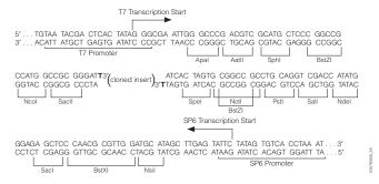
Figure 1. The promoter and multiple cloning sequence of the pGEM®-T Vector. The top strand corresponds to the RNA synthesized by T7 RNA polymerase. The bottom strand corresponds to the RNA synthesized by SP6 RNA polymerase.
